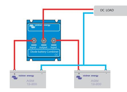
System with two batteries
